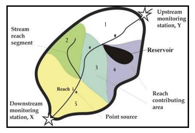
Total Load at X = L1+L2+L3+L4+L5Incremental Load at X = L5 only
